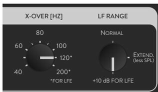
For the use in LFE channel set-ups the BASS subwoofers can be set to LFE, the preferred format for film sound reproduction. The Format means a 120 Hz crossover point and an additional + 10 dB level.
